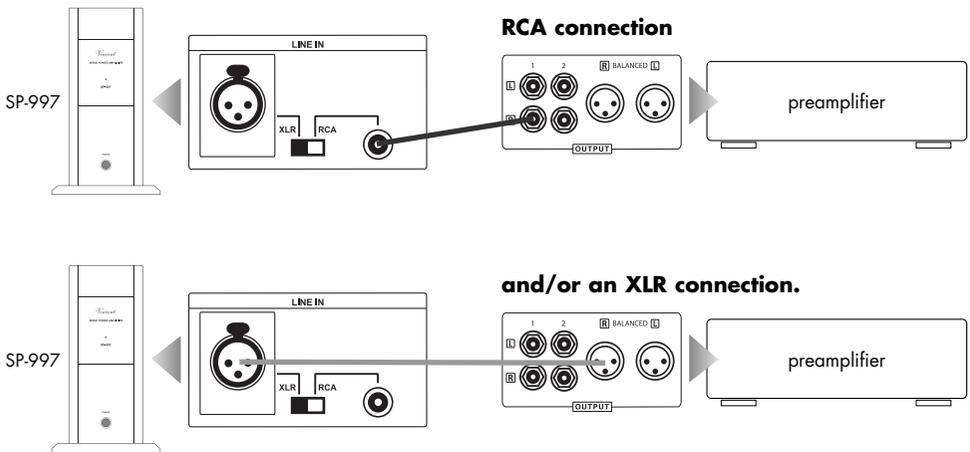
Both "LINE IN" inputs can be connected to preamplifiers at the same time and in this way it is possible to connect two preamplifiers simultaneously and toggle between the inputs. Make sure the volume of the respective preamplifier is not set too high before switching.
