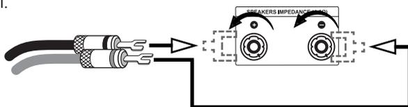
If no connector is to be used, remove approximately 1 cm length of insulation from each end of the speaker wire. Twist the braid in order to avoid short circuits. Turn the fastener on the loudspeaker terminal counter clockwise to loosen it and introduce the bare wire end into the exposed connector hole. Then turn the fastener clockwise so that the wire is firmly clamped. Make sure the connection is pretty tight.
