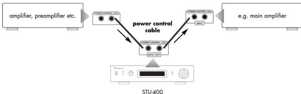
A theoretically infinite number of devices may be served with the switch impulses from a transmitting device. To this end, on most devices one of the two "POWER CONTROL" connectors may be used as a signal input and the other as a signal output. This method of passing on the signal via the devices' inputs and outputs and of thereby chaining them is also known as "daisy chaining".
