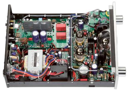
Despite high component density, there are no thermal problems with the tubes.
